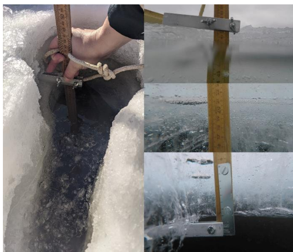
Ice gauge in use (left) and as seen under water (right).
