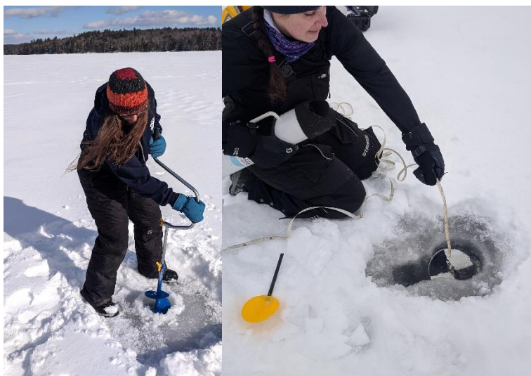
Maggie with ice auger (left) and fitting Secchi disk through expanded ice hole (right).
