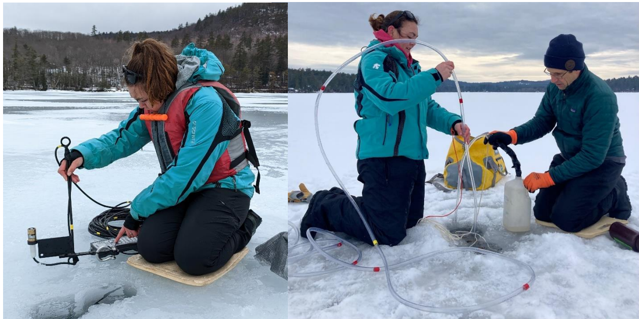
Shannon measuring light above the ice on Keoka Lake (left) and using a core tube with Ben to collect water samples on Woods Pond (right).
