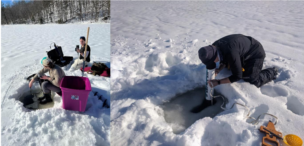
Maggie using the sonde and handheld data logger and Shannon using the light meter on Middle Pond (left) and Maggie measuring Secchi depth on Keyes Pond (right).
